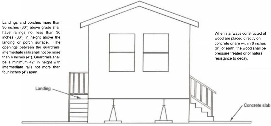
If an exit door swings outward in the direction of travel, a landing must be provided. The landing surface may not be more than 1 inch (1") below the bottom opening of the doorway. The landing width and length must not be less than the width of the door.
